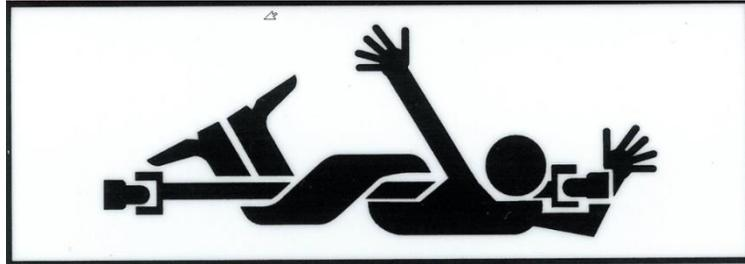
Never use your hands to clear if clogged. Never allow anyone to reach into the rotor housing. The rotor can crush and/or dismember. Keep everyone clear of the rotor until the prime mover engine is off and the hydraulic pressure has been relieved.
