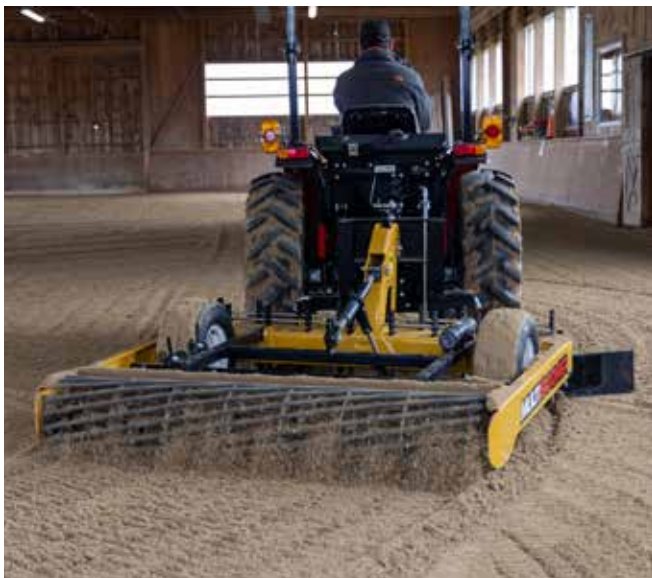
Multi-Groomer shown with optional board scraper and swivel hitch.
